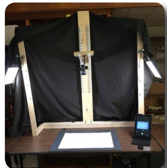
Figure 3: PCS Prototype constructed of wood.
